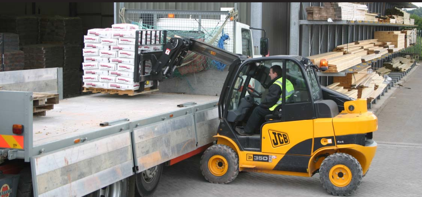
Efficient use of space, a perfect example. This Builder's Merchant delivery lorry is parked so it does not obstruct access to the warehouse (left) or the timber racking (right). The TLT 35D 4 x 4 is placing a 1.6 tonne pallet of cement bags to the far side.
